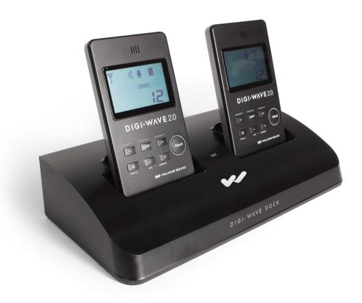
NEW! The Digi-Wave Dock offers an innovative extension to the Digi-Wave two-way wireless communication system from Williams Sound. It provides a simple, flexible way to connect portable Digi-Wave systems to other fixed systems. The connection begins when a Digi-Wave transceiver or receiver is simply plugged into the Dock. The Dock provides continuous power and/or charging for two Digi-Wave devices, and has separate audio inputs and outputs in each of its bays.
